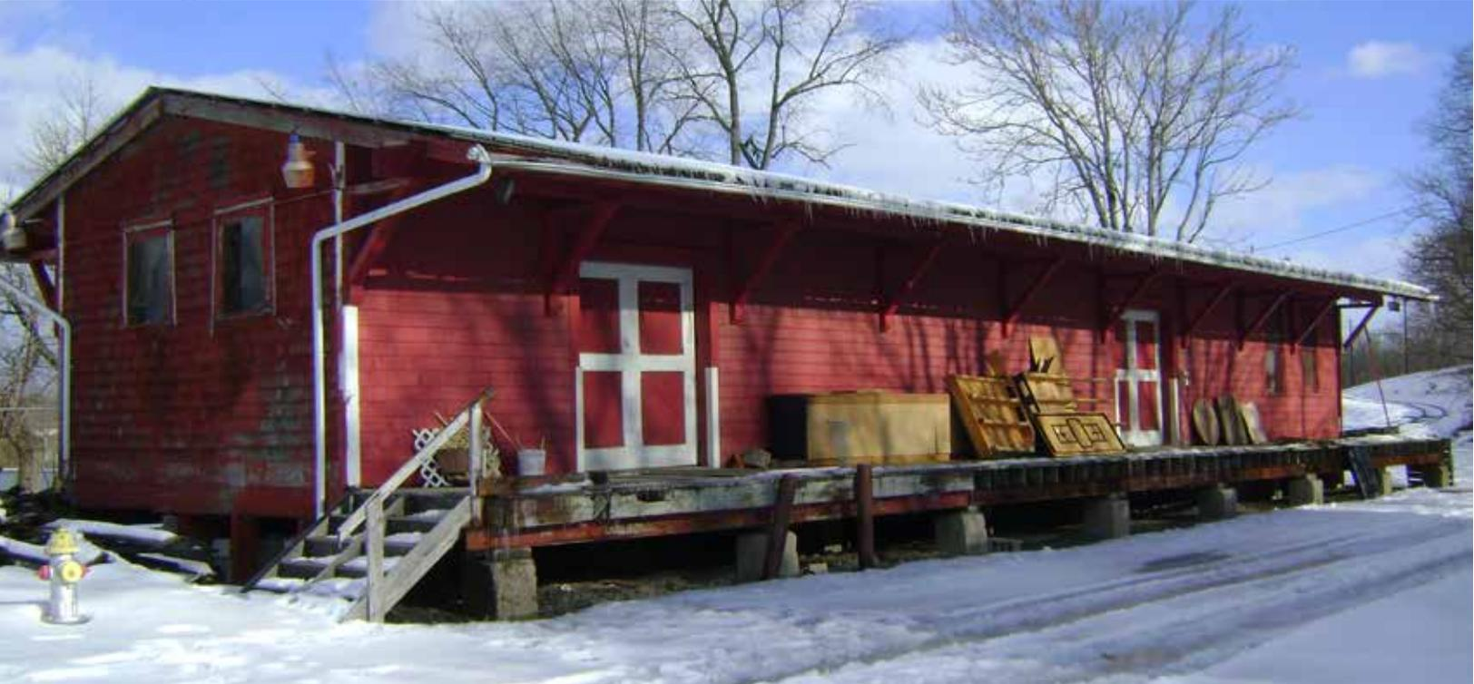
The wide overhanging eaves of the side gable roof sheltered the platforms and the station doors from the elements. The building's architectural elements included exposed rafters, triangular knee braces, and wood shingle siding.
